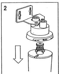
**STEP 1.** Turn cartridge slowly, approximately 90° counterclockwise until it hits a stop and the slot on the cartridge lines up with the word "OFF" on the head. At this position the inlet and outlet ports have been closed and the filter internal pressure has been relieved.
