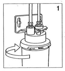
Replace cartridge when there is a decided decrease in water flow or when objectionable taste and/or odors return. It is recommended that the cartridge be CHANGED AT LEAST EVERY SIX MONTHS. ALWAYS HAVE SPARE CARTRIDGES ON HAND.
