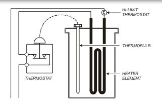
Fig. 5 Heat Control Diagram
