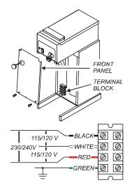
Fig. 3 115/240 Volt Terminal Block
