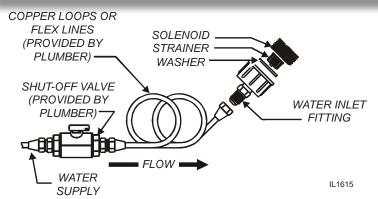
Fig. 2 Water Supply Installation
