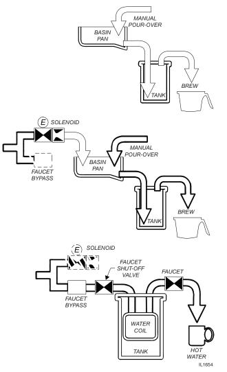
Fig. 6 Water Flow Diagram
