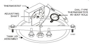
Fig. 10 Checking and Adjusting Brew Temperature
