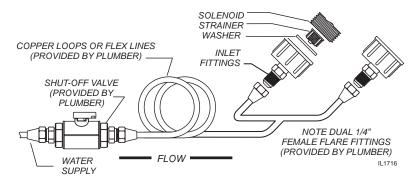
Fig. 2 Water Supply Installation
