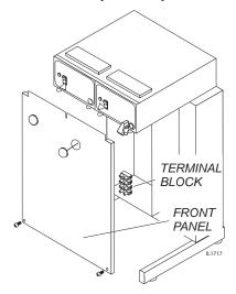
Fig. 3 115/230 Volt Terminal Block
