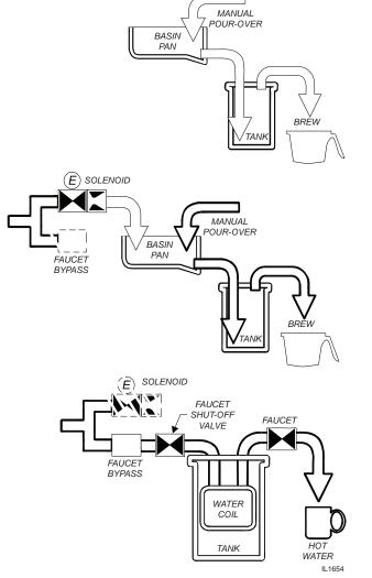
Fig. 6 Water Flow Diagram
