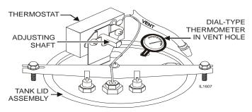
Fig. 10 Checking and Adjusting Brew Temperature
