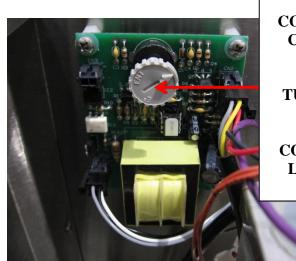
TO ACCESS HEATER CONTROL, REMOVE REAR COVER WITH MACHINE UNPLUGGED.
